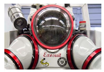
Developed and built in North Vancouver by **Nuytco Research Ltd**, this hard metal dive suit allows divers to operate safely down to a depth of 1000 feet and yet still have exceptional dexterity and flexibility to perform delicate work. The amazing technology of the **EXOSUIT** atmospheric diving system (ADS) maintains a cabin pressure of the surface and still allows the suit to bend due to a unique rotary joint invented by Dr. Phil Nuytten.
