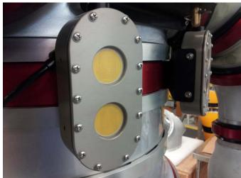
The NewtSun 100 replaces and improves upon a 500W halogen or 150W discharge lamp. These lights are virtually impervious to shock, maintenance free, and have a life expectancy of 50,000 hours.
