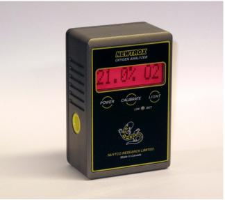
**Nuytco**'s second generation oxygen analyzer is microprocessor-based to ensure consistent calibration. Developed specifically for use in Nuytco submersibles and in the Exosuit, it features:
