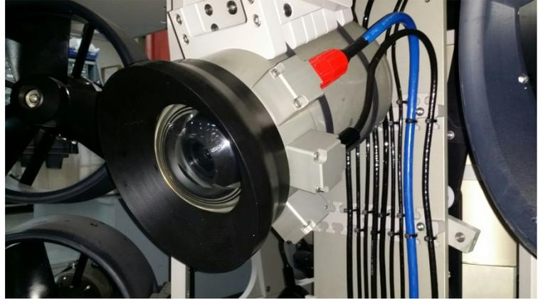
Fiber optic and electronic multiplexers are not only expensive, they are limited in their number of available channels. Nuytco has addressed this problem with its ultra-low latency, over network camera, which has a staggering glass to glass delay of only 46m seconds. Because the video is served over your network, you're only limited by bandwidth – on a 10Gbps uplink that that equates to 70+ HD, or 35+ 4K cameras!
