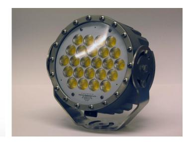
Producing an unheard of 65,000 Lumens, with a CRI of 80 and colour temperature of 5000K, the NewtSun 500 has little competition. The NewtSun 500 body is milled from 6061T6 aluminum billet and hard anodized.
