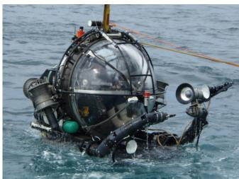
The one-atmosphere **Deep Rover** is a 3300ft (1000m) depth-rated, one person submersible. Two 64" acrylic hemispheres offer panoramic viewing. Deep Rover's incredible viewing dome, two five-function manipulators with 5' reach, HD camera and lighting arrays make Deep Rover an extremely versatile platform.
