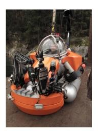
The one-atmosphere **DeepWorker 2000** submersible allows a pilot to go deeper and spend more time below the surface than traditional diving methods. The compact and lightweight **DeepWorker 2000** is easy to operate and can be piloted with minimal training. Horizontal and vertical thrusters give unparalleled manoeuverability; the **DeepWorker 2000** can hover and 'fly' underwater.
